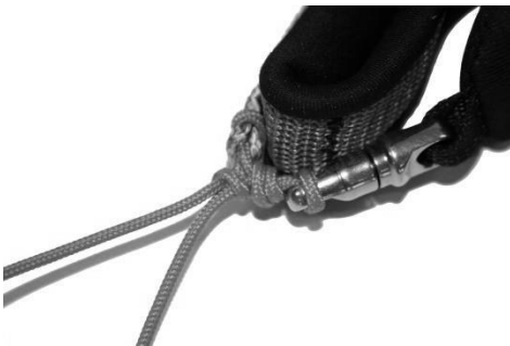
Fig. 8 Knot on the brake handle
