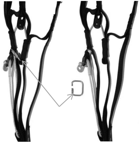
Fig. 13 MITO riser with and without speed limiter
